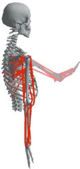
Fig. 11. Muscle paths are generated as Catmull-Rom splines through muscle origin, insertion, and via points
