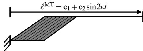
**Fig. 4 Schematic of the musculotendon actuator used in the elastic-tendon and rigid-tendon computational benchmarks. In the simulations, the initial length of the musculotendon actuator was set to  $c_1 = \ell_s^T + \ell_o^M \cos \alpha_o$  and then the length was varied by  $c_2 \sin 2\pi t$ .**
