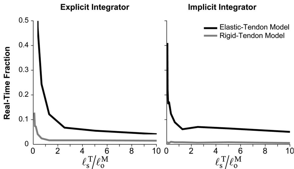
**Fig. 8 Computational speed of the damped equilibrium (black curve) and rigid-tendon (gray curve) musculotendon models as functions of tendon slack length ( $\ell_s^T$ ) normalized by the optimal fiber length ( $\ell_o^M$ ) using explicit (left) and implicit (right) integrators. Wall clock time was divided by the amount of time simulated to obtain the real-time fraction; values below 1 indicate that the simulations completed faster than real time.**
