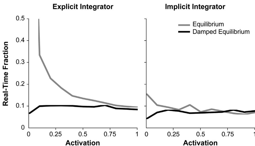
**Fig. 6** Time required to generate the simulation results shown in Fig. 5 using explicit (left) and implicit (right) integrators. Wall clock time was divided by the amount of time simulated to obtain the real-time fraction; values below 1 indicate that the simulations completed faster than real time.
