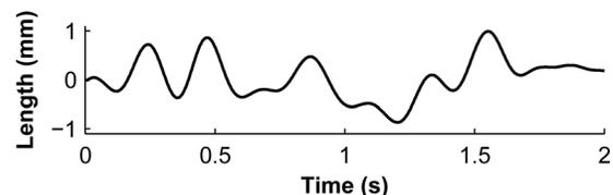
**Fig. 11** Waveform of the change in musculotendon length [30] used in the submaximal-activation biological benchmark, shown here with a maximum length change of 1.0 mm. This waveform was scaled by the appropriate maximum length change (either 1.0 mm or 8.0 mm), added to  $\ell_s^T + \ell_o^M \cos \alpha_o - 4$  mm, and then used to prescribe the displacement of the free end of the tendon.
