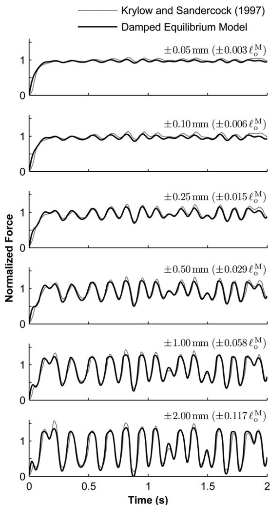
**Fig. 10** Comparison of experimental [29] (gray curve) and simulated (black curve) force profiles from maximally-activated muscle undergoing length changes of maximum amplitude 0.05 (top), 0.1, 0.25, 0.5, 1.0, and 2.0 mm (bottom). The maximum isometric force used in the model was  $f_o^M = 1.27$  N and the optimal fiber length was  $\ell_o^M = 17.1$  mm.
