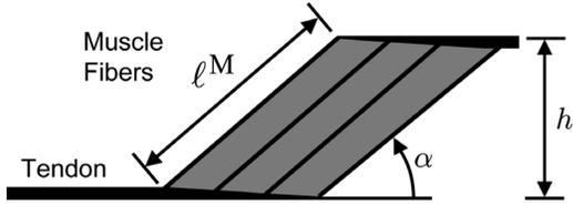
**Fig. 1** Simplified geometric representation of muscle fibers and tendon for musculotendon modeling. Muscle fibers are assumed to be straight, parallel, of equal length, coplanar, and attached to tendon at a pennation angle ( $\alpha$ ). As the muscle shortens, the distance  $h$  remains constant and the pennation angle increases. Adapted from Zajac [23].
