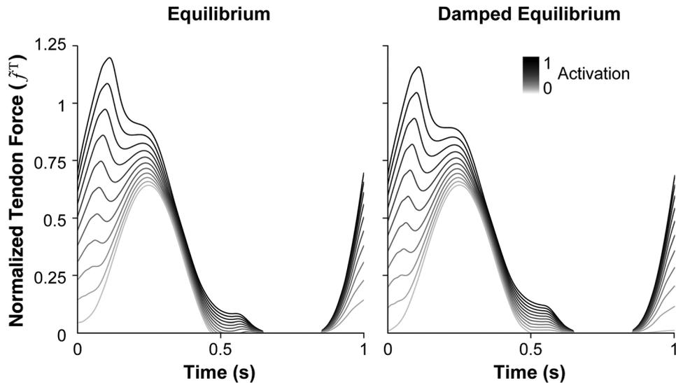
**Fig. 5** Normalized tendon force profiles of the equilibrium (left) and damped equilibrium (right) musculotendon models. Each muscle underwent constant-activation, sinusoidal-displacement simulations of 1-s duration with activations varying from 0 (0.01 for the equilibrium model) to 1 in increments of 0.1. The average absolute difference between normalized force profiles generated by the models was less than 0.3% at low activation and less than 2.5% at high activation.
