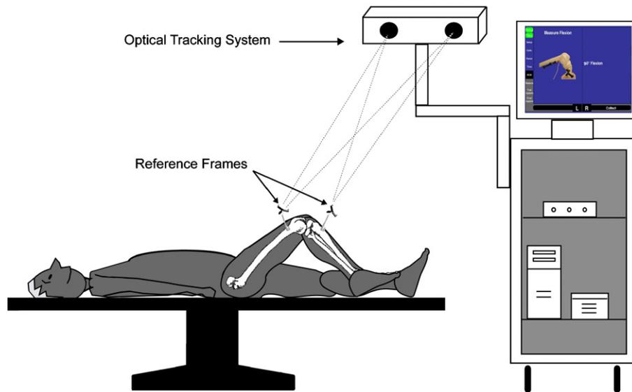
Fig. 1. Components of an image-free navigation system. The optical tracking system measures the position and orientation of reference frames that are attached to the patient's femur and tibia. Information such as cut plane orientation and limb alignment is displayed on the computer monitor.
